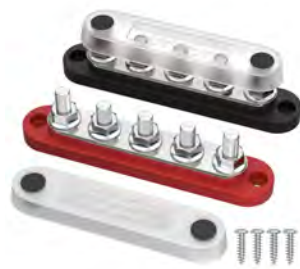
DBB004 RD BK 120AAC/150A DC, 300V AC/48V DC 5*M6(1/4") Terminal Studs L106mm*W23mm*H28.5mm
