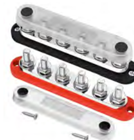
DBB018 RD BK 300A 300V AC, 48V DC 6*M10(3/8") Studs L178mm*W37.8mm xH43.2mm
