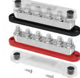
DBB022 RD BK 600A 300V AC/48V DC 6*M10(3/8") Studs L178mm*W37.8mm xH53.2mm
