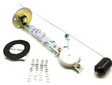
FCS02-7810 Float Style Sending Unit 78-100OHM, 5-27" Adjustable
