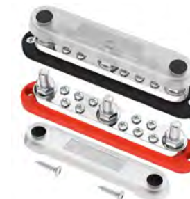
DBB017 RD BK 300A 300V AC/48V DC 3*M10(3/8")+10*M4(#8) L178mm*W37.8mm*H43.2mm
