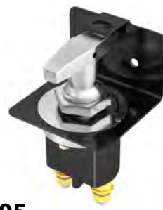
SS205 ON-OFF Switch 2*M10(3/8") Studs Continuous(Amp):500A Crank(Amp):5000A Voltage:12-24VDC
