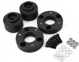
LELK005 Leveling Lift Kit 3" Front&1.5" Rear Fit Dodge Ram 1500 4WD 2WD
