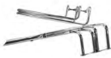
EHD510 CH BK PL CA Universal Fit Small Block Chevy V8 Roadster Shotgun Headers
