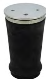
ASB220 Universal Air Spring Bag 93mmX121mm 3/8"-16 Fastener, Range 109mm~250mm
