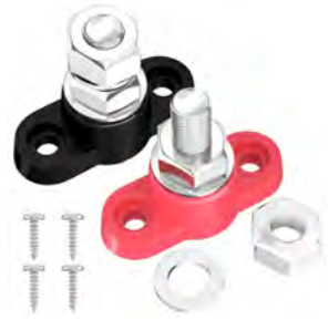
DBB001 RD BK 80A DC 48VDC, 300V AC/48V DC M8(5/16")/M10(3/8") Studs L53mm*W25.5*H41.5mm
