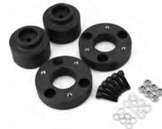
LELK006 Leveling Lift Kit 3" Front&2" Rear Fit 2009-2021 Dodge Ram 1500 4WD 2WD
