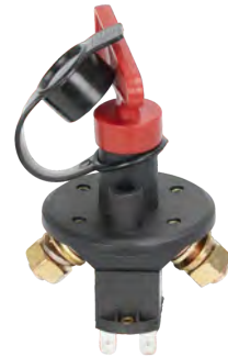
SS203 ON-OFF Switch 2*M10(3/8") Studs Continuous(Amp):200A Crank(Amp):1000A Voltage:12-24VDC
