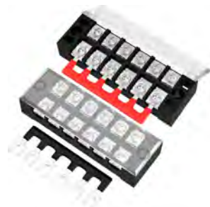
DBB026 RD BK 600V 35A Terminal Block 12mm Space, 6 Position with Cover L91.5mm*W30mm*H19mm
