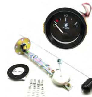
SENDER12K Float Style Sending Unit Kits w/52mm Fuel Level Gauge
