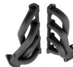
EHD591 CH BK PL CA 1964-73 Mustang, 1966-73 Falcon Small Block Ford 260-302 Shorty Headers
