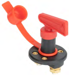
SS201 ON-OFF Switch 2*M10(3/8") Studs Rating:300A 60VDC Voltage:12-24VDC Installing:4x40mm
