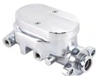
BRMC02F GM Chrome Master Cylinder Finned Top 1" Bore 9/16 & 1/2" Dual Sided Ports
