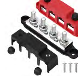
DBB023 RD BK 300A 300V AC/48V DC 4*M8(5/16") Studs L138mm*W69mm*H35mm
