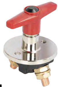
SS204 ON-OFF Switch 2*M10(3/8") Studs Continuous 200A, Crank 1000A Voltage:12-24VDC Installing:2x40mm
