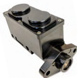
BRMC03 Universal Billet Alum Master Cylinder 1" Bore 9/16 & 1/2" Ports Black, Chrome, Polish
