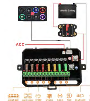
SWP008 8 Gang Switch Panel System with Silicone waterproof
