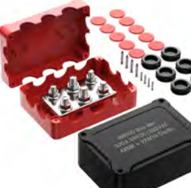
DBB021 RD BK 500A 300V AC/48V DC 6*M8(5/16") Studs L124mm*W86mm*H46.5mm
