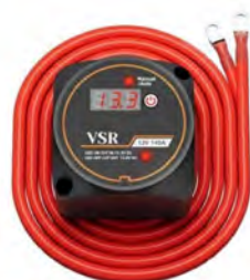
RLS009 Smart Dual Battery Isolator 12V 140A With Manual Control Button LED ON Cut in 13.3VDC LED OFF Cut out 12.8VDC
