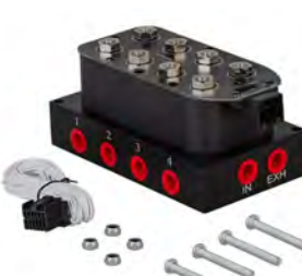
SVAL006 Universal 12V Manifold Solenoid Valve 8*1/4 NPT Output & 4*1/8 NPT Inlet
