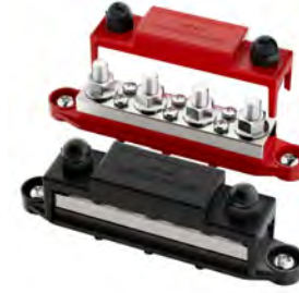
DBB024 RD BK 400A 300V AC, 48V DC 4*M10(3/8") Studs+6X#10 Screw L165mm*W33.8mm*H46.2mm
