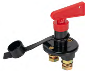
SS202 ON-OFF Switch 2*M10(3/8") Studs Rating:300A 60VDC Voltage:12-24VDC Installing:2x40mm
