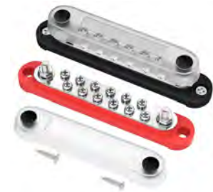
DBB005 RD BK 120AAC/150A DC, 300V AC/48V DC 2*M6(1/4") Studs+12*M4(#8) Screw L150mm*W28mm*H35mm
