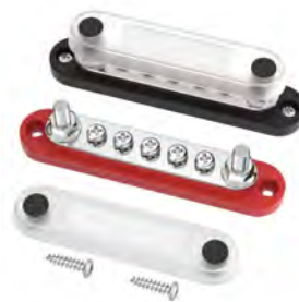
DBB003 RD BK 120AAC/150A DC, 300V AC/48V DC 2*M6(1/4") Studs+5*M4(#8) Screw L106mm*W23mm*H28.5mm
